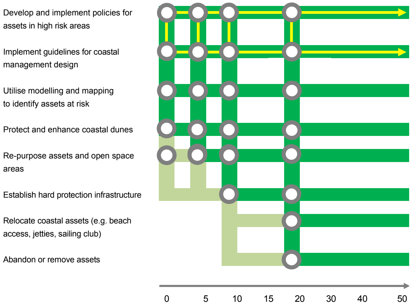
Figure 14. Adaptation pathway for built coastal assets on Kangaroo Island. Refer Attachment D for legend and explanation of adaptation pathways.
