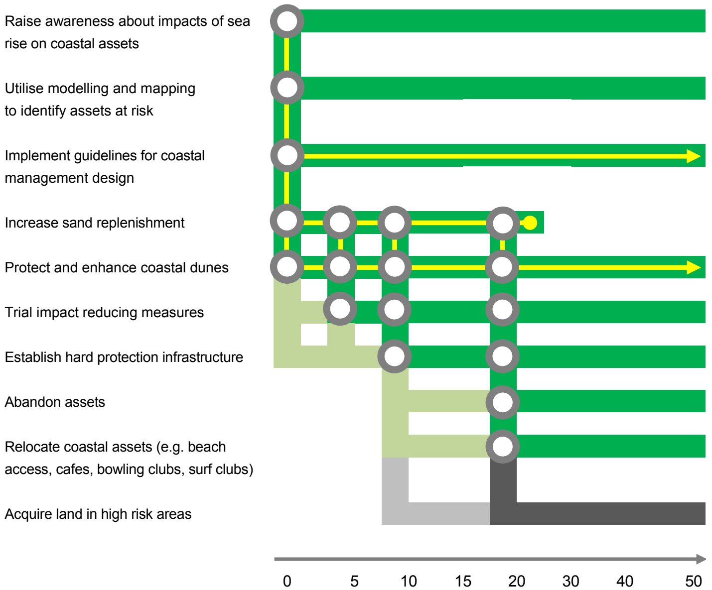
Figure 10. Adaptation pathway for built coastal assets on the Fleurieu Peninsula.
